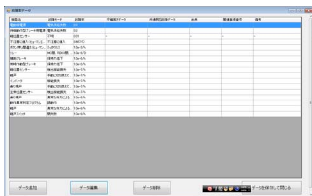
Fig. 6 Component failure data window.
