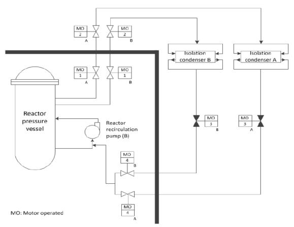
Fig. A4 Schematic of Isolation Condenser (IC) [A4-1]
