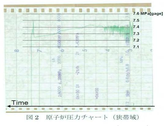
Fig. A10-1 Chart of the reactor pressure (narrow band)
