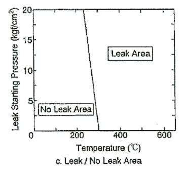
Fig. A10-2 The relation between the pressure and the heatproof temperature of the silicone rubber. [A10-3]
