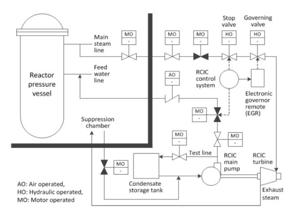
Fig. A5 Schematic of Reactor Core Isolation Cooling System (RCIC) [A5-2]
